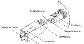
X1 Positive Terminal Note: When wiring, do not apply exessive force to X1 and X2
